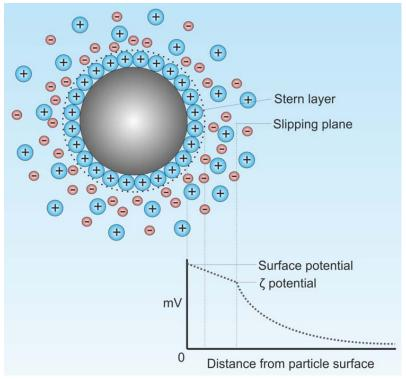
This diagram shows a graph of the potential difference as a function of distance from the surface of a particle suspended in a dispersion medium.
